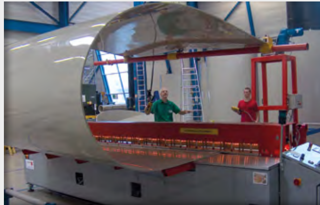
Sheet rolling unit K-ZV for sheet thicknesses between 6 - 30 mm and diameters between 1000 - 5,000 mm (only in conjunction with overhead crane)
