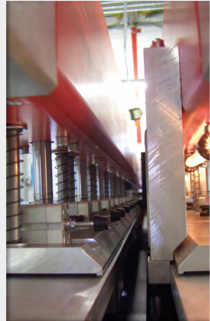
Automatic 90° L-welding device (option for butt welding machines), e.g. in order to produce rectangular tanks
